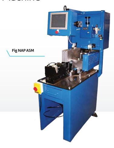
Complete cutting equipment system for small sizes  $\frac{3}{4}$ " – 2" pipe, fabrication machine utilizes a cold saw.
